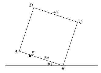
A uniform square lamina ABCD of side 4a and weight W rests in a vertical plane with the edge AB inclined at an angle  $\theta$  to the horizontal, where  $\tan \theta = \frac{1}{3}$ . The vertex B is in contact with a rough horizontal surface for which the coefficient of friction is  $\mu$ . The lamina is supported by a smooth peg at the point E on AB, where BE = 3a (see diagram).
