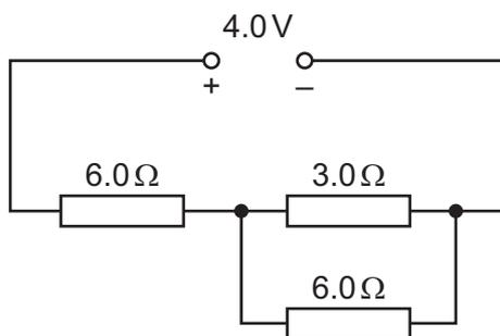
The potential difference (p.d.) across the network is  $4.0\text{V}$ .
