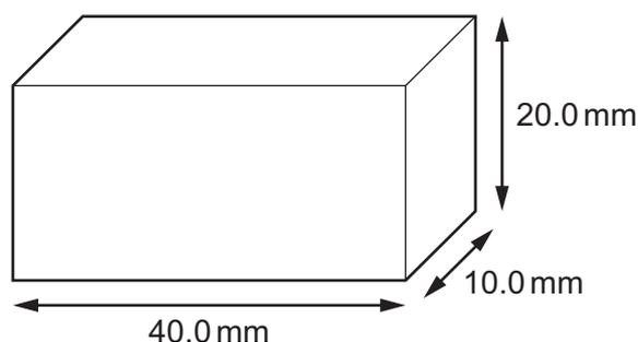
The calipers can measure with an absolute uncertainty of  $\pm 0.1$  mm.
