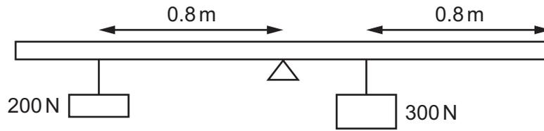
Weights are hung from two points on the bar as shown in the diagram. To maintain equilibrium, a couple is applied to the bar.
