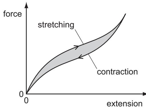
The force–extension curve for contraction is below the force–extension curve for stretching.
