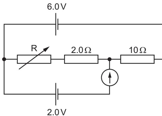
The cell of electromotive force (e.m.f.) 6.0V has negligible internal resistance. A cell of e.m.f. 2.0V and a galvanometer are connected into the potential divider. The resistance of R is varied until the galvanometer reads zero.
