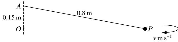
A particle  $P$  of mass  $0.3 \text{ kg}$  is attached to a fixed point  $A$  by a light inextensible string of length  $0.8 \text{ m}$ . The fixed point  $O$  is  $0.15 \text{ m}$  vertically below  $A$ . The particle  $P$  moves with constant speed  $v \text{ m s}^{-1}$  in a horizontal circle with centre  $O$  (see diagram).
