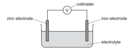
The zinc electrode dissolves in the electrolyte forming Zn<sup>2+</sup>(aq) ions.
