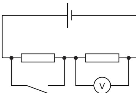
When the switch is open the voltmeter reads 1.5 V.
