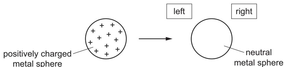
What happens to the charges on the neutral sphere as the positively charged sphere is brought close to it?
