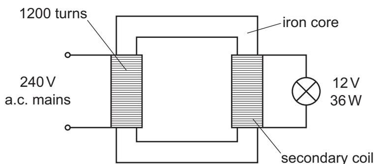
Which row shows the number of turns in the secondary coil and the current in the mains wires?
