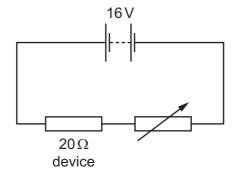
What is the resistance of the variable resistor when the power dissipated in the electrical device is 4.0 W?
