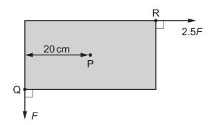
Two forces act in the plane of the board. Force F acts at corner Q and force 2.5F acts at corner R. The perpendicular distance between the line of action of force F and point P is  $20\,\mathrm{cm}$ . The board is in equilibrium.
