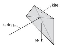
The kite has three forces acting on it: the weight W, the tension T in the string, and the force F from the wind.
