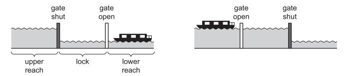
Boats are raised and lowered in the lock as the level of water changes. When the lock is 'full' it contains 150 000 litres of water; when it is 'empty' it contains just 50 000 litres.
