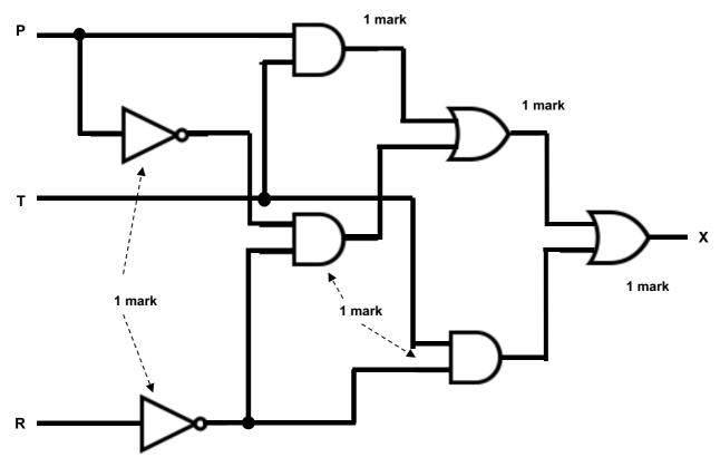
Note: input T has 2 cross overs that should not be connections
