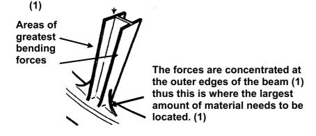
(ii) Joists in a building structure. [1]
