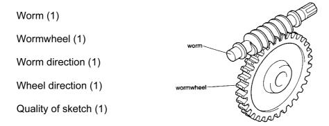
(ii) The VR of the system is large (1) as the worm (driven gear) has effectively one tooth (1). [2]
