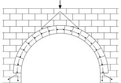
(b) (i) Strain gauge 1 will measure tension [1] Strain gauge 2 will measure compression [1] [2]
