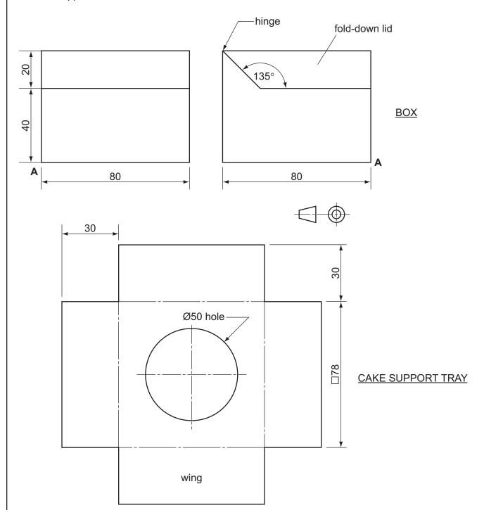
In the space to the right, draw a full-size isometric view of the cake box with the cake support tray in position. The lid is to be shown fully open in the vertical position. The starting point for corner **A** has been given for you. [10]
