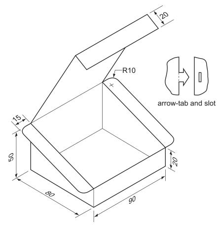
The box uses arrow-tabs and slots to join the sides together.
