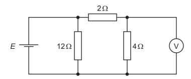
The voltmeter has a very high resistance and reads a potential difference  $V_{\text{out}}$ .
