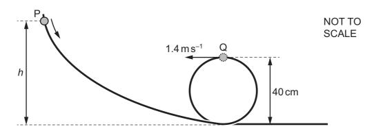
The track loops around and forms a vertical circle of diameter 40 cm. At point Q, the bead has a speed of  $1.4\,\mathrm{m\,s^{-1}}$ .
