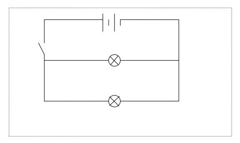
(ii) electricity can still flow through the other lamps/still a complete circuit through the other lamps;
