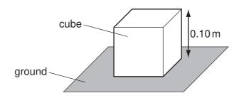
The cube weighs 200 N and its sides are 0.10 m long.
