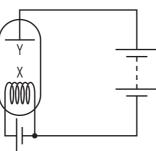
Which particles are emitted in the diode, and from where are they emitted?
