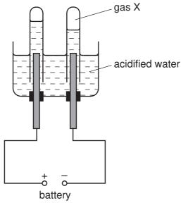
Gas X ignites with a pop when tested with a lighted splint.
