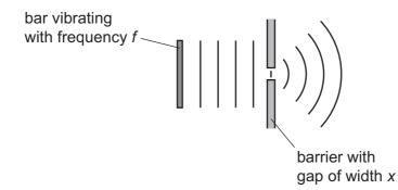
The waves pass through a gap of width *x* in a barrier so that diffraction occurs.
