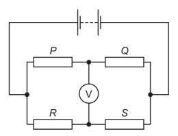
The voltmeter reading is zero.
