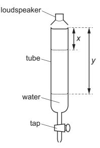
A tap at the bottom of the tube is opened so that water slowly leaves the tube. For some lengths of the air column in the tube, the sound heard is much louder.
