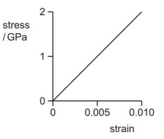
What is the strain energy per unit volume of a rod made from this metal when the strain of the rod is 0.010?
