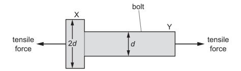
The bolt has a circular cross-section. At end X the diameter is 2*d*. At end Y the diameter is *d*.
