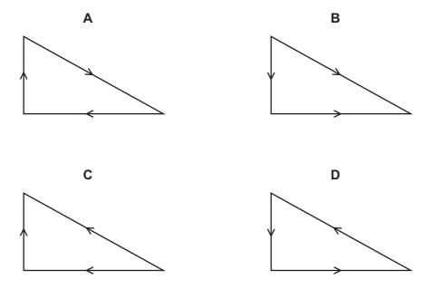
**14** Two rigid steel beams XY and YZ are fixed at their lower ends and are hinged at Y. Each beam is inclined at 50° to the horizontal, as shown. A weight of  $4.0 \times 10^4$  N hangs from Y. The structure is in equilibrium.
