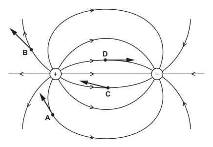
32 Lightning can occur between a charged cloud and the Earth's surface when the electric field strength in the intervening atmosphere reaches 25 kN C<sup>-1</sup>. The diagram shows the electric field between the base of a cloud and the Earth's surface.
