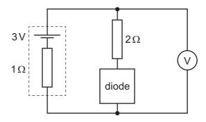
A high-resistance voltmeter is connected across the diode and resistor.
