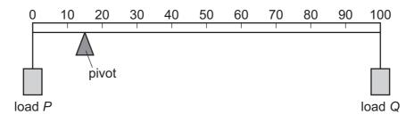
Which combination of pivot position and loads causes the beam to be in equilibrium?
