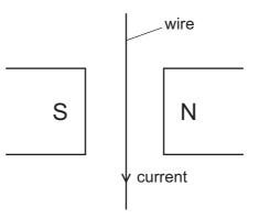
The magnet and current cause a force to act on the wire.
