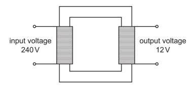
What is a possible pair of values for the number of turns in the primary coil and the number of turns in the secondary coil?
