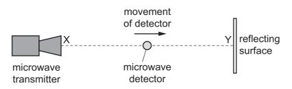
A microwave detector is moved steadily in a straight line from X to Y. A series of maxima and minima of intensity is obtained. The distance between adjacent maxima is 1.5 cm.
