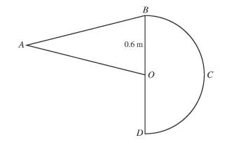
A uniform lamina *OABCD* consists of a semicircle *BCD* with centre *O* and radius 0.6 m and an isosceles triangle *OAB*, joined along *OB* (see diagram). The triangle has area  $0.36 \text{ m}^2$  and AB = AO.
