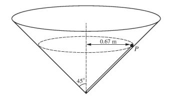
A particle P is moving inside a smooth hollow cone which has its vertex downwards and its axis vertical, and whose semi-vertical angle is 45°. A light inextensible string parallel to the surface of the cone connects P to the vertex. P moves with constant angular speed in a horizontal circle of radius 0.67 m (see diagram). The tension in the string is equal to the weight of P. Calculate the angular speed of P. [6]
