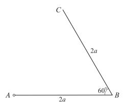
Two uniform rods AB and BC, each of length 2a and mass m, are rigidly joined at B so that angle  $ABC = 60^{\circ}$  (see diagram). The system is free to rotate in a vertical plane about a horizontal axis though A. Show that the moment of inertia of the system about this axis is  $\frac{14}{3}ma^2$ . [3]
