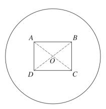
A uniform circular disc has radius  $0.5 \,\mathrm{m}$ , centre O and mass per unit area  $6.20 \,\mathrm{kg} \,\mathrm{m}^{-2}$ . A rectangle ABCD, where AC and BD intersect at O, is removed (see diagram). The lengths of AB and BC are  $0.4 \,\mathrm{m}$  and  $0.3 \,\mathrm{m}$  respectively. Show that the moment of inertia of the resulting lamina, about an axis through A perpendicular to its plane, is  $0.851 \,\mathrm{kg} \,\mathrm{m}^2$ , correct to 3 significant figures. [8]
