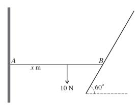
A light rod AB of length 0.8 m has a particle of weight 10 N attached to a point at a distance x m from A. The rod rests in equilibrium in a horizontal position with A against a rough vertical wall and B on a smooth plane inclined at  $60^{\circ}$  to the horizontal (see diagram). Find, in terms of x, the magnitude of the force that the inclined plane exerts on the rod.
