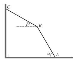
Two uniform rods AB and BC, each of length 2a and mass m, are smoothly hinged at B. They rest in equilibrium with C in contact with a smooth vertical wall and A in contact with a rough horizontal floor. The rods are in a vertical plane perpendicular to the wall. The rods AB and BC make angles  $\alpha$  and  $\beta$  respectively with the horizontal (see diagram). Show that
