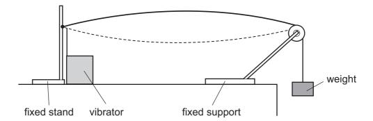
A vibrator is attached to the wire near the clamped end. A stationary wave with one loop is produced. The frequency of the vibrator is *f*.
