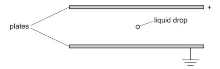
A small charged liquid drop, midway between the plates, is held in equilibrium by the combination of its weight and the electric force acting on it.
