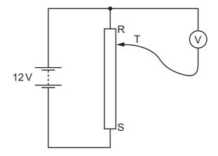
As the sliding terminal T is moved from R to S, what happens to the reading on the voltmeter?
