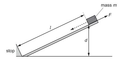
As the box slides down the slope, it loses gravitational potential energy and it does work against the friction.
