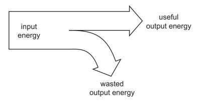
The device is 50% efficient.
