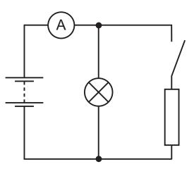
With the switch open, the ammeter reads 2.4 A. When the switch is closed, this reading increases to 4.0 A.
