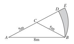
The diagram shows an isosceles triangle ABC in which AB = 8 m, BC = CA = 5 m. ABDA is a sector of the circle, centre A and radius 8 m. CBEC is a sector of the circle, centre C and radius 5 m.
