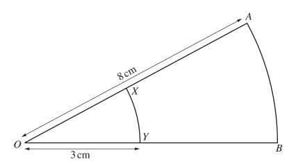
The diagram shows a sector OXY of a circle centre O, radius 3 cm and a sector OAB of a circle centre O, radius 8 cm. The point X lies on the line OA and the point Y lies on the line OB. The perimeter of the region XABYX is 15.5 cm. Find
