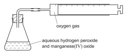
$40\,\mathrm{cm^3}$  of aqueous hydrogen peroxide was put in the flask and 0.1 g of small lumps of manganese(IV) oxide was added. The volume of oxygen collected was measured every 30 seconds. The results were plotted to give the graph shown below.
