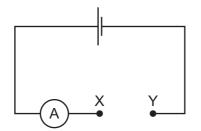
Four wires of different length and thickness are connected in turn between point X and point Y. All four wires are made of the same metal.
