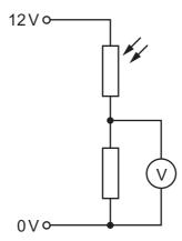
The light falling on the light-dependent resistor (LDR) increases in brightness.
