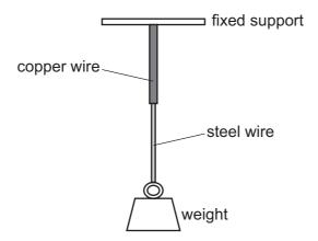
The combination wire is stretched by a weight added to its end. Both the copper and the steel wires obey Hooke's law.
