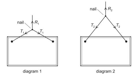
In both cases, a string is attached to the same points on the picture and looped symmetrically over a nail in a wall. The forces shown are those that act on the nail.
