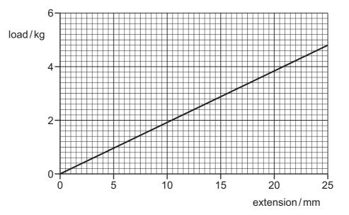
How much work is done on the wire to increase the extension from 10 mm to 20 mm?
