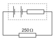
The current in the resistor is 40 mA for a time of 60 s. During this time 6.0 J of energy is lost in the internal resistance.
