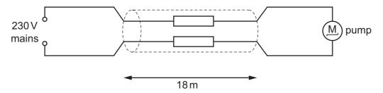
The performance of the pump is acceptable if the potential difference (p.d.) across it is at least 218 V. The current through it is then 0.83 A.
