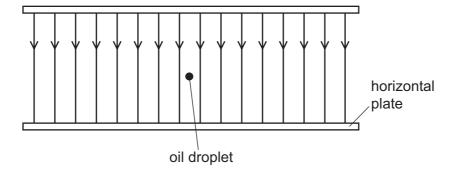
The weight of the droplet is exactly balanced by the electrical force on the droplet.
