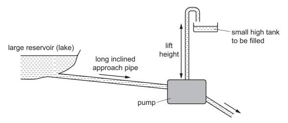
In one such pump the long approach pipe holds  $500\,\mathrm{kg}$  of water. A valve shuts when the speed of this water reaches  $2.0\,\mathrm{m\,s^{-1}}$  and the kinetic energy of this water is used to lift a small quantity of water by a height of  $15\,\mathrm{m}$ .
