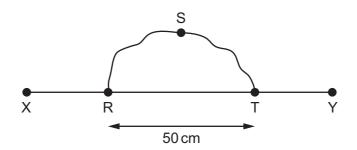
Each wire is  $100 \, \text{cm}$  long with a resistance per unit length of  $10 \, \Omega \, \text{m}^{-1}$ .
