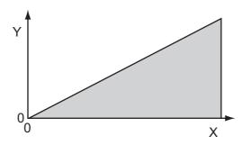
The shaded area represents the total strain energy stored in stretching the wire.
