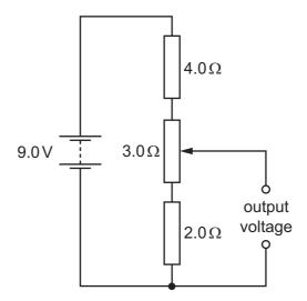
What are the maximum and the minimum output voltages of this potential divider circuit?
