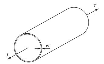
The tube is under tension, caused by a force T, parallel to the axis of the tube. To reduce the stress in the material of the tube, it is proposed to thicken the wall.
