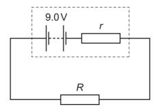
A charge of 6.0 C flows through the resistor in a time of 2.0 minutes causing it to dissipate 48 J of thermal energy.
