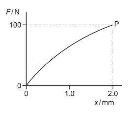
What could be the value of the strain energy stored in the wire when it is stretched elastically to point P?
