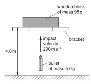
A bullet of mass 5.0 g is shot vertically upwards into the wooden block of mass 95 g. It embeds itself in the block. The impact causes the block to rise above its supporting brackets.
