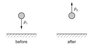
The ball has momentum  $p_1$  downwards just before hitting the ground. After rebounding, the ball leaves the ground with momentum  $p_2$  upwards. The ball is in contact with the ground for 0.020 s. During this time interval, an average resultant force of 25 N acts on the ball.
