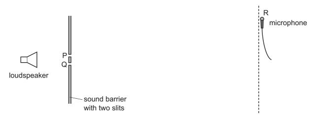
What is the condition for an intensity maximum (loud sound) to be detected by a microphone at R?
