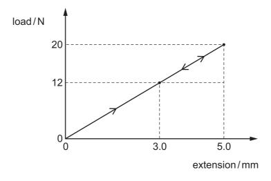
How much strain energy is released during the unloading process?
