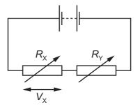
The variable resistors have resistances  $R_X$  and  $R_Y$ .  $V_X$  is the potential difference across resistance  $R_X$ .
