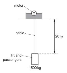
The lift and passengers have a combined mass of 1500kg. The motor raises the lift through a distance of 20 m.
