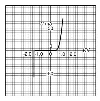
What is the resistance of the diode for applied potential differences of +1.0 V and -1.0 V?
