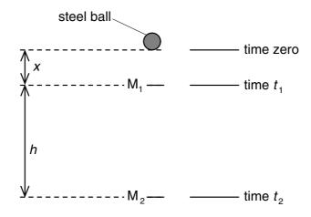
When a steel ball is released from rest from a point a distance x above M<sub>1</sub>, it is found that the ball takes time  $t_1$  to reach  $M_1$  and time  $t_2$  to reach  $M_2$ .
