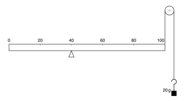
At which mark on the rule must a 50 g mass be suspended so that the rule balances?
