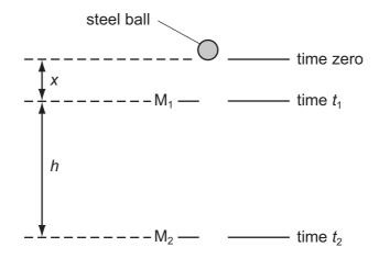
A steel ball is released at time zero from a point a distance x above  $M_1$ . The ball reaches  $M_1$  at time  $t_1$  and reaches  $M_2$  at time  $t_2$ . The acceleration of the ball is constant.
