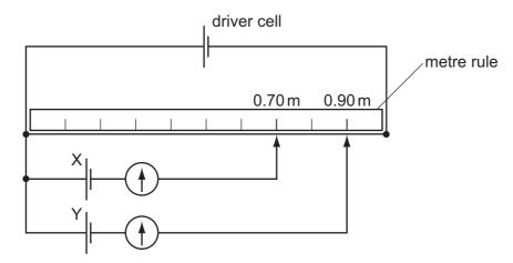
The balance points for cells X and Yaradre 0.0907 despectively. If the e.m.f. of cell, Xwhiast list the e.m.f. of cell Y? A 0.609 B 0.806 C 0.909 D 1.44
