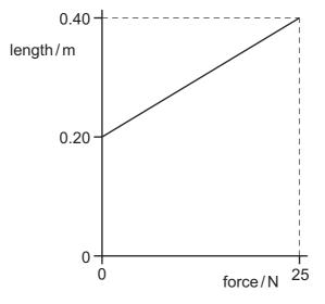
What is the maximum strain energy in this deformed rubber cord?
