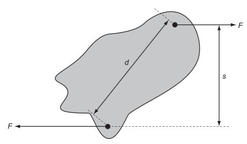
What is the magnitude of the torque on the body produced by these forces?
