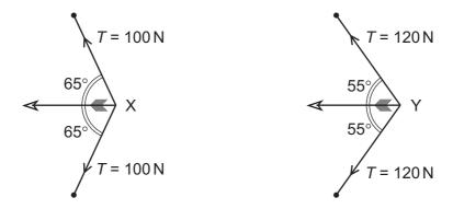
The resultant force on the arrow is greater when the arrow is released from position Y.
