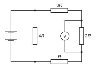
The voltmeter reading is 2V.
