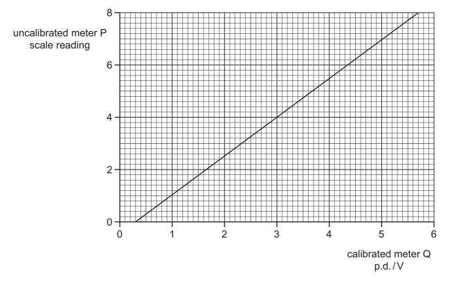
The graph shows that meter P has a zero error. This meter is now adjusted to remove this zero error. When the meter is recalibrated, the gradient of the calibration graph is found to be unchanged.
