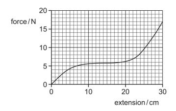
What is the best estimate of the strain energy stored in the rubber band when it is extended 30 cm?
