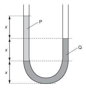
What is the ratio  $\frac{\text{density of P}}{\text{density of Q}}$ ?
