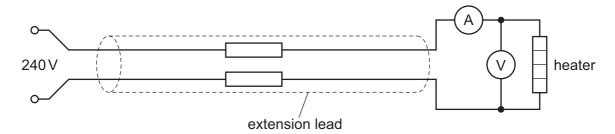
A voltmeter measures the potential difference (p.d.) across the heater as 216 V and an ammeter measures the current through the heater as 7.7 A.
